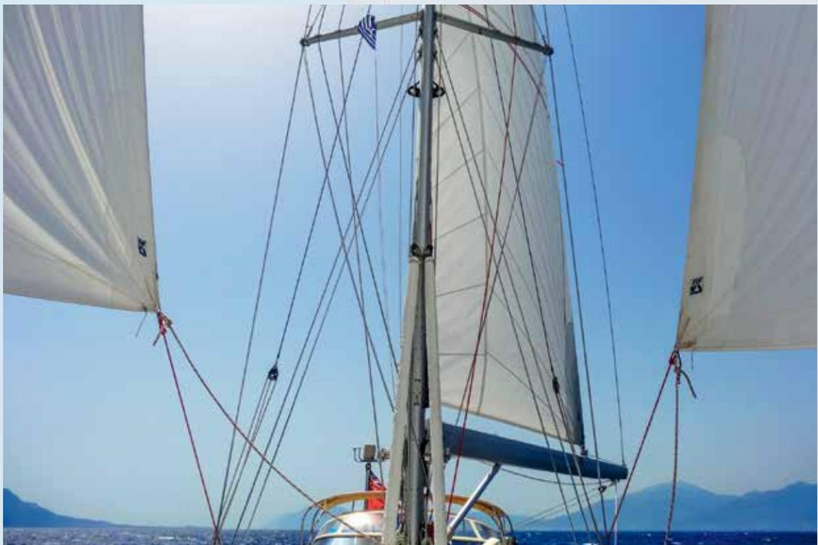
LEFT: The twin headsail arrangement – where identical jibs are attached to a single furler section – simplifies downwind sailing, particularly for short-handed crews.
