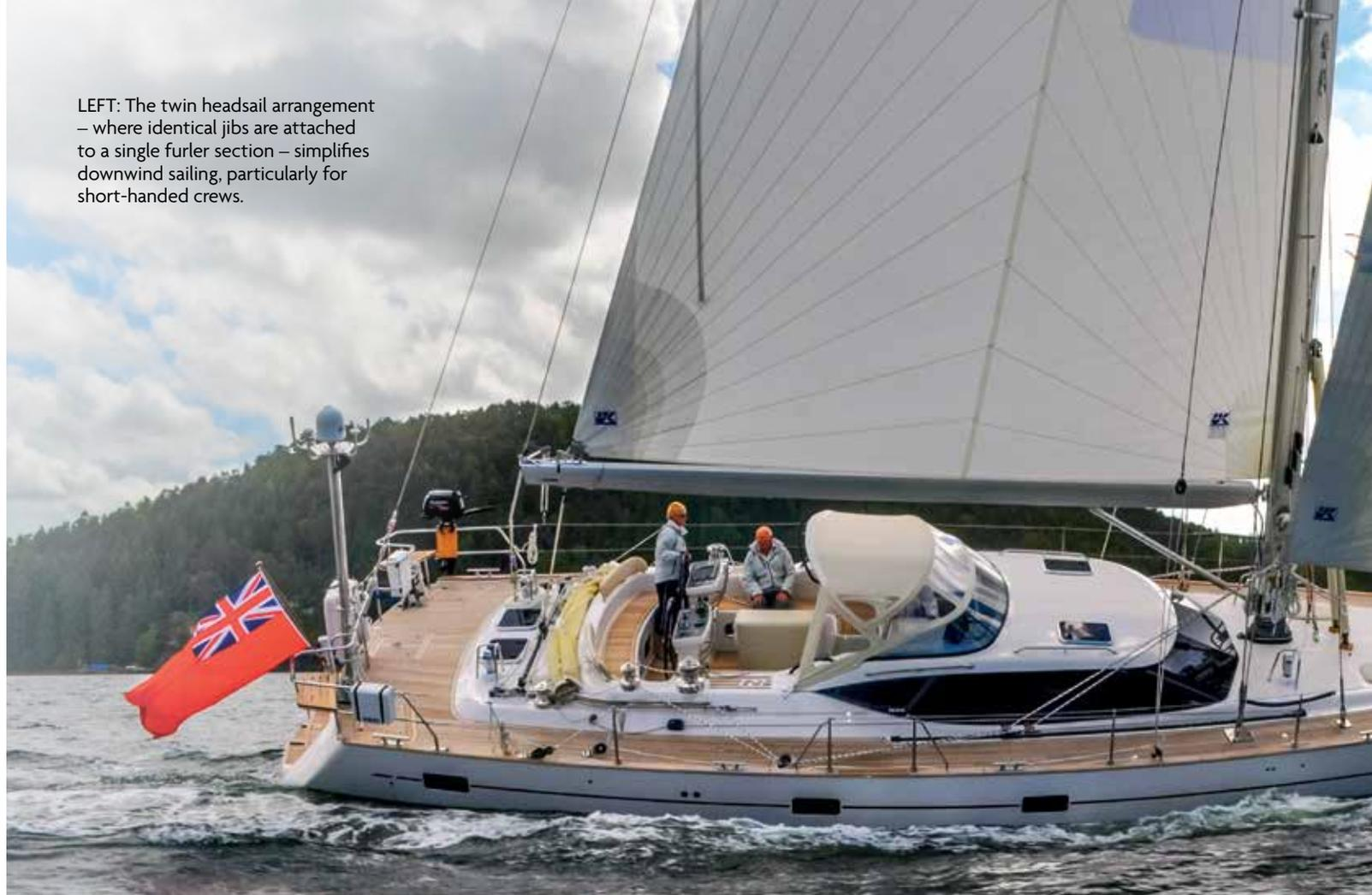
the windward jib. The accumulated wind is redirected into the leeward jib which would otherwise be blanketed by the mainsail. To gybe, simply haul and release the mainsheet onto the new tack leaving the whisker poles and jib sheets unaltered.
