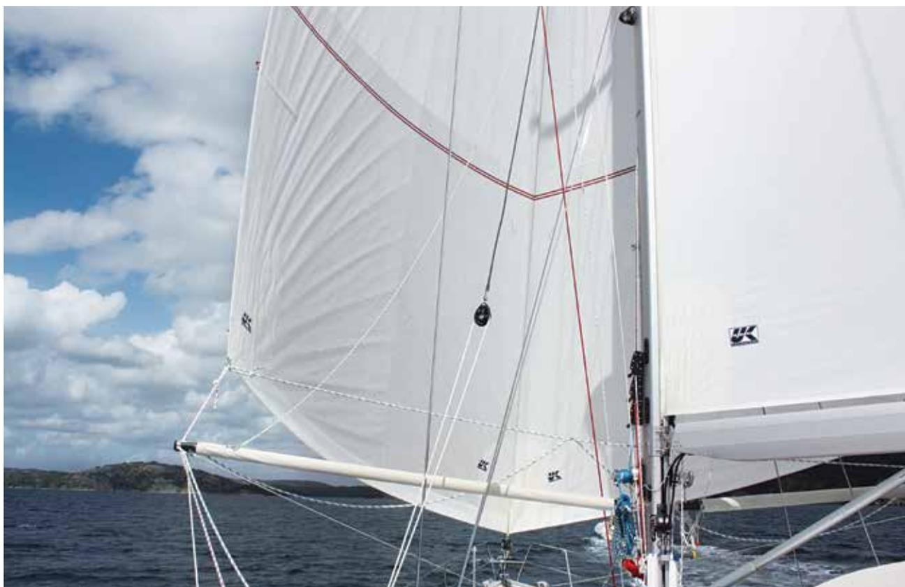
makers, the twin jibs can be partially furled or reefed, or completely struck. One person can control the Simbo rig entirely from the cockpit in all weather conditions. The only time it's necessary to go forward is to raise or lower the whisker poles.
