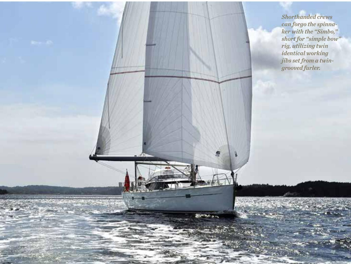
*Shorthanded crews can forgo the spinnaker with the “Simbo,” short for “simple bow” rig, utilizing twin identical working jibs set from a twin-grooved furler.*
