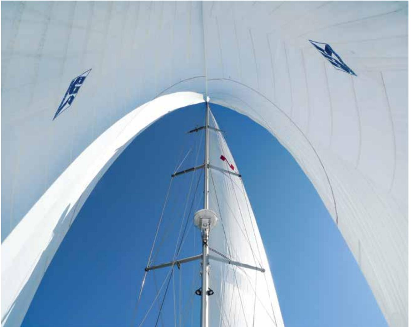
run, the wind flows into the mainsail, on around the mast into the weather jib, and is then deflected into the leeward jib (that would otherwise have been blanketed by the mainsail). When jibbing, overhaul the mainsheet and jibe the mainsail as you normally would. Everything else — the jib sheets, the separated twin jibs, the whisker poles and guys — remains in place.
