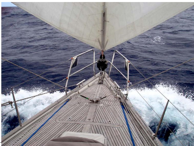
Running downwind, showing the forward pole guys
