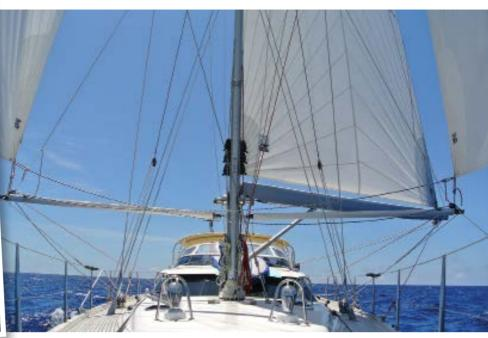
ABOVE: Side view shows how the rig does not encroach on the mast.
