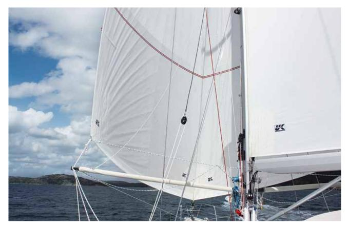
nakers, the twin jibs can be partially furled or reefed, or completely struck. One person can control the Simbo rig entirely from the cockpit in all weather conditions. The only time it's necessary to go forward is to raise or lower the whisker poles.
